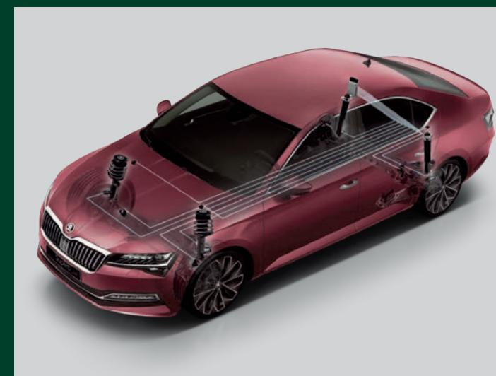
Dynamic Chassis Control with Drive Mode Selector (DCC)
